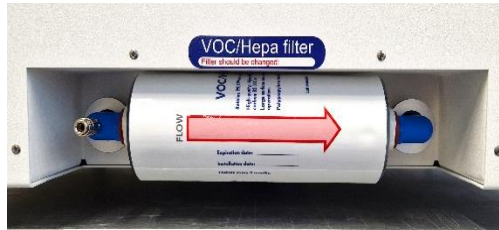
Figure 12.3 Filtre VOC/HEPA correctement installé
